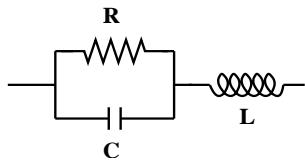
$$|Z| = \frac{1}{\sqrt{1 + (RC\omega)^2}} \sqrt{R^2 + (L\omega(1 + (RC\omega)^2) - (R^2C\omega))^2}$$
